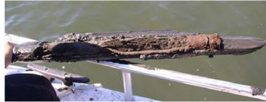
Figure 5 Soil sample collected with a McCauley/Eijkelkamp peat sampler.
