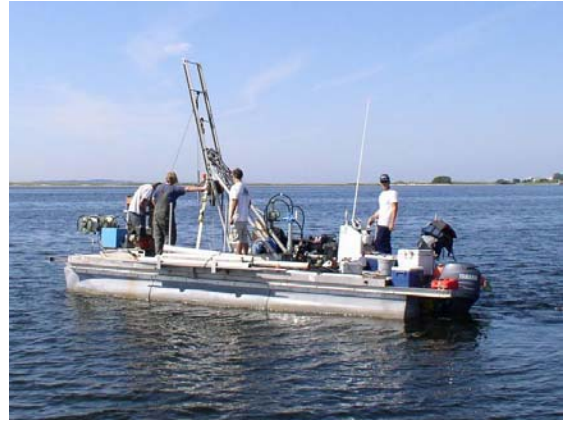
Figure 6 University of Rhode Island Graduate School of Oceanography vibracoring vessel in Little Narragansett Bay.
